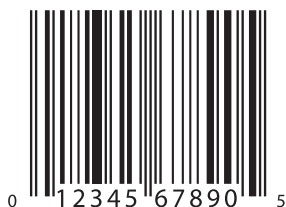
Figure 4 UPC-A Bar Code Symbol
