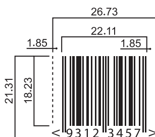
Figure 20 EAN-8 Bar Code Symbol at Nominal Size (100%)
