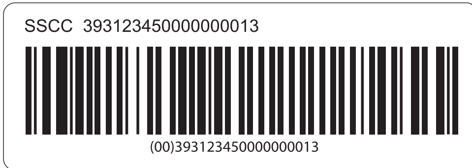
Figure 13 The Basic Logistics Label : An SSCC
