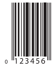
Figure 5 UPC-E Bar Code Symbol
