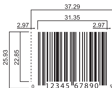
Figure 21 UPC-A Bar Code Symbol at Nominal Size (100%)
