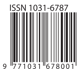
Figure 9 EAN-13 Bar Code Symbol Formed Using the ISSN
