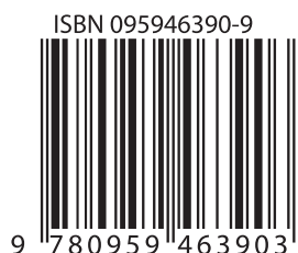
Figure 8 EAN-13 Bar Code Symbol Formed Using the ISBN
