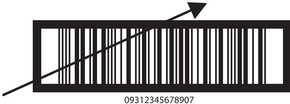
Figure 25 Example of a Skewed Scanning Beam
